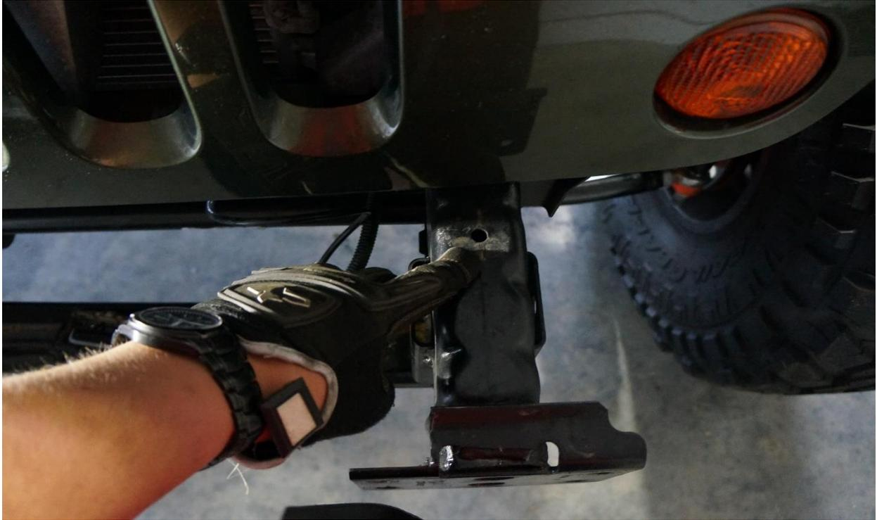
Once these are drilled, slide bumper over the frames and insert one of the  $\frac{1}{2}$ "x5  $\frac{1}{2}$ " bolts into each of the back two mounting holes on the bumper through the holes you just drilled out to  $\frac{1}{2}$ ".
